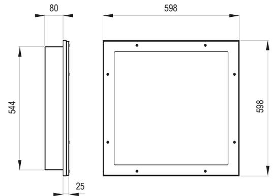
**Square recessed body manufactured from zinc coated steel with upstand recess.**
