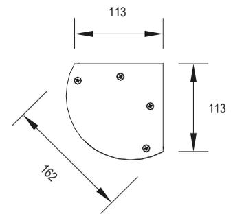
**Angled LED fitting with a slim-line curved profile capable of continuous mounting (cable runs can be housed within angled back body).**
