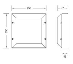
Square bulkhead developed with LED at the forefront of its design, combining high performance, strength and durability.
