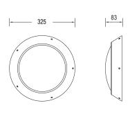
Round bulkhead developed with LED at the forefront of its design. With an impact rating of IK20 it is extra, extra strong and is conceivably the strongest vandal resistant fitting on the market. Aluminium spun body with steel bezel.
